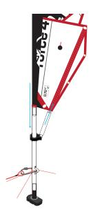
Erect the mast and make sure the stays are secure, then carefully slide the mast into the vertical mast sleeve on the sail, holding the boom spigot upright and threading this into the boom sleeve as the sail approaches it. The previously fitted boom should slide into the boom spigot as the sail settles down the mast.
