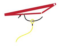
Tie a double overhand stopper knot in one end of the length of bungee, thread this through one of the eyelets in the bottom of the sail and through the nylon rope thimble fitted to one end of mainsheet.
