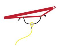
Thread the bungee through the other eyelet in the bottom of the sail before tying another double overhand stopper knot.
