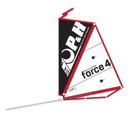
Take the boom (sold separately as part of the Mast & Rig Kit) and feed it flattened end first into the horizontal boom sleeve at the bottom of the sail, until the flattened end engages in the plastic fitting which caps this sleeve.
